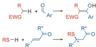
**Scheme 5.** Organocatalyzed reactions that can be switched on and off. Top: aldol type additions of C–H acids (EWG = electron-withdrawing group) to carbonyl compounds (with catalysts from Scheme 1 and 3). Bottom: Michael additions of thiols to unsaturated carbonyl compounds (with catalysts from Scheme 2 and Scheme 4).
